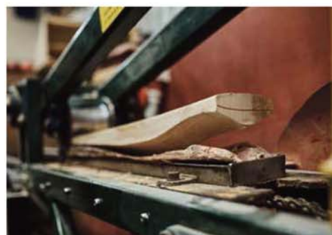
On the press is another clue to Dan's engineering past; rather than using old bits of carpet to rest the blade level, as witnessed in many bat factories, we find a carbon fibre mould to hold the blade in place. Each model in the range has its own custom mould to fit its specific shape.
