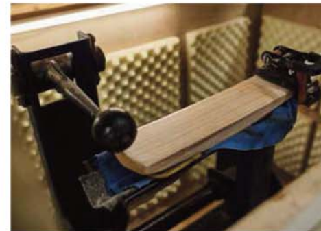
This knocking-in device in its soundproof box is in constant use. Designed by Dan, this bespoke machine provides the equivalent of five hours of knocking-in by hand in a fraction of the time. This unique bit of kit is a real feather in the cap for Chase with every bat made getting strapped in for preparation.
